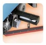
The waste collection hopper (15 l.) and the brushes can be easily removed without the use of tools
